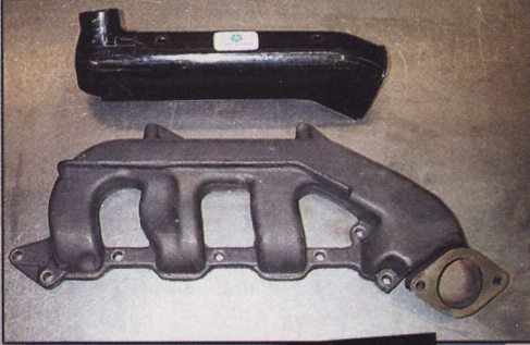
JOHN PORTED THE UNIQUE EXHAUST MANIFOLDS FOR OPTIMUM PERFORMANCE
