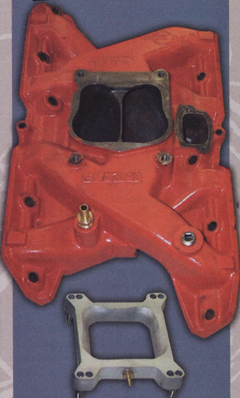
DESPITE BEING ORIGINALLY DESIGNED FOR A SPREAD BOARD THERMOQUAD, JOHN USED AN ADAPTER TO RUN AN 800 CFM HOLLEY FOR MORE HORSE POWER.
