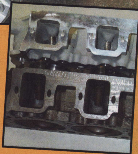
The port sizes of the A148 are staggering! (shown on lower head) The intake ports are 4.28 square inches, up from 3.51 inches.
